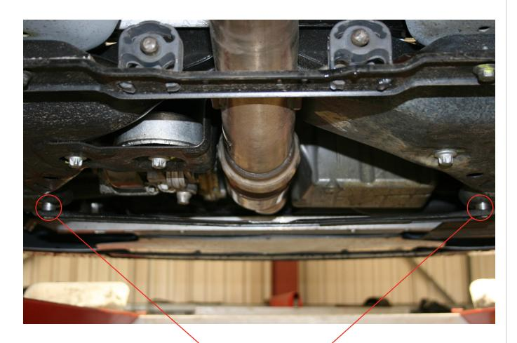
`Attach 10mm spacers ' using original bolts
